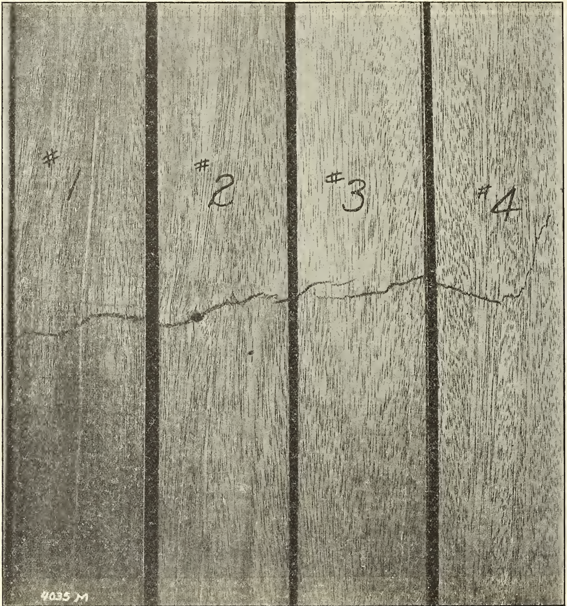
Fig. 17.—Influence of compression failure occurring during growth on failures in static bending. African mahogany.
